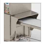
A fixed large cover is installed to ensure a safe distance. The outfeed conveyor is equipped with a connection detection sensor. This prevents
