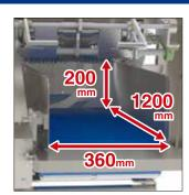
The feed tank has a size of W360\*H200\*L1200m m. It can hold up to two batches of products. Productivity is improved with a slice speed of 300 shots per minute.
