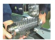
Belt attachment and removal can be performed quickly and easily.
